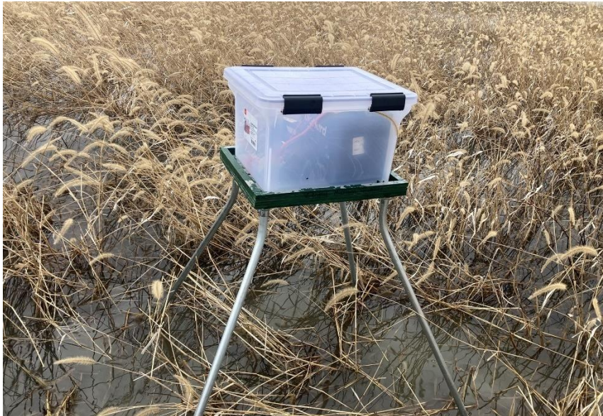
Figure A1. An audio playback station used to broadcast rail calls overnight.
